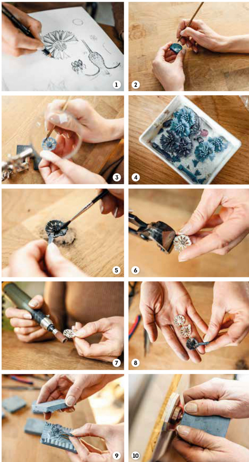
1/CORNFLOWER STUDY The shape of leaves, front and profile view, proportions of the individual parts. 2/ WAX First, the flower is carved out of hard jewellery wax. 3/ UNDER THE LENS The softest details need to be fine-tuned under the magnifying glass. 4/WASTE If a leaf falls off, the process begins anew. 5/ CHARCOAL The wax model is blackened out to reveal any details in need of fine-tuning. 6/ GATE CLIPPING Large pincers for tiny blossoms. 7/ GRINDER Grinding and polishing makes the silver's beauty pop. 8/ COMPARISON The wax model and silver castings, before and after processing. 9/RUBBER MOULD The first silver model is moulded in rubber, resulting in a mould for making new flowers. 10/ HOT WAX The mould is filled with high-pressure hot wax to create another flower which is then cast using the lost-wax casting method.
